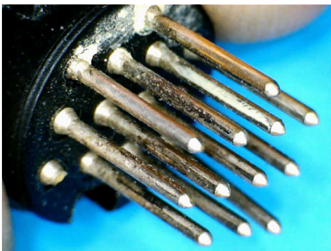
8 YEAR OLD 13-PIN UN-PROTECTED PLUG Including broken pin
